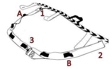
The shoulder strap can be adjusted in 6 positions by varying the loop on which the terminal carabiner is attached. In the image, with the letter "A" is identified the loop intended for operators with lower stature. With the letter "B", is identified the loop suitable for operators with higher stature. Each intermediate position, correspond to a variation of operator's height of about 5cm.
