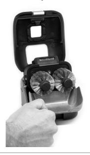
Remove the solder collection tray for disposal of solder waste.
