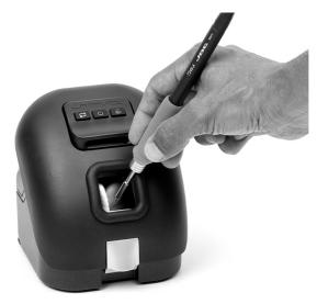
The CLMU-A is automatically switched off if the splashguard is opened during operation.
