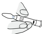
4.3 Carefully remove the polyethylene sealing. Ensure that the powdery reagent contained in the cap does not fall out.
