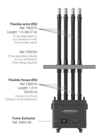
In this configuration aspiration at stand is not available, aspiration flow is set High. Note that in this configuration, suction force per intake is decreased when compared to 2 work intakes configuration (see details on page 14). Change Work intakes parameter into 4 in order to set this configuration (see page 7).
